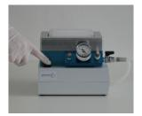
Push the "START" button and filtration starts automatically
