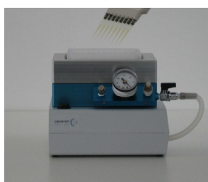
Pipette sample into the filter plate
