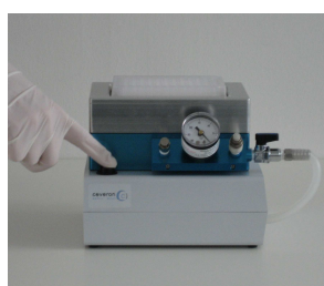
Push the "START" button and filtration starts automatically
