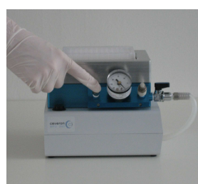
After filtration is terminated push the "VENTILATION" button
